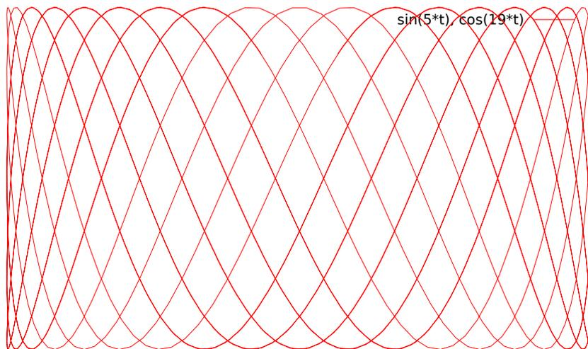
Lissajou Curve generated with respect to parameters May, 19th
